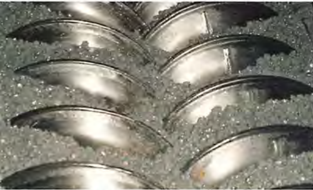
The Holo-Flite's unique intermeshing screws are ideal for many difficult drying applications.
