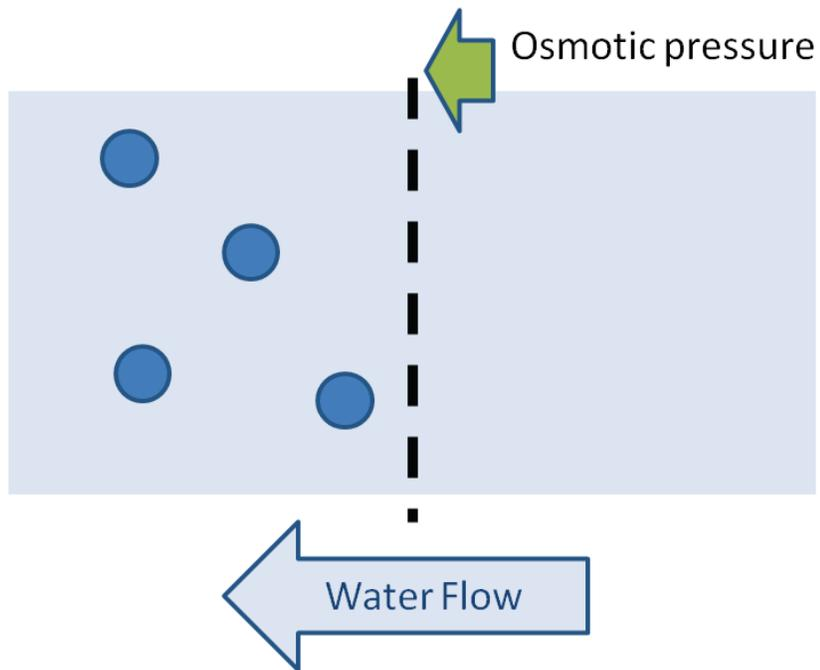
**Figure 11.1:** When fresh and salty water are separated by a semi-permeable membrane (which lets water through but not salt ions), the water will flow from the fresh side to the salty side. In this picture, the light blue background is supposed to represent the water and the blue circles indicate the salt ions.
