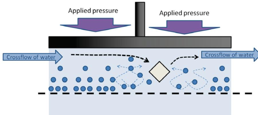
**Figure 11.5:** The crystals of limescale formed will disturb the concentration layer so that more of the ions that have built up are washed away, the concentration near the membrane is reduced and the flow rate is increased.
