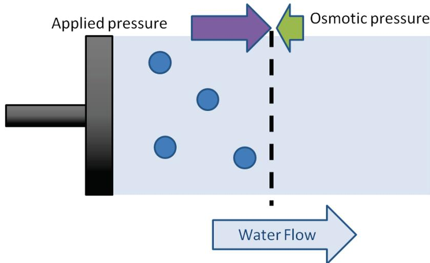
**Figure 11.2:** If the pressure on the salty side is increased enough then water can be forced in the reverse direction, from the salty side to the fresh side. The ions cannot pass through the membrane, so the water that has been passed through is made salt-free.
