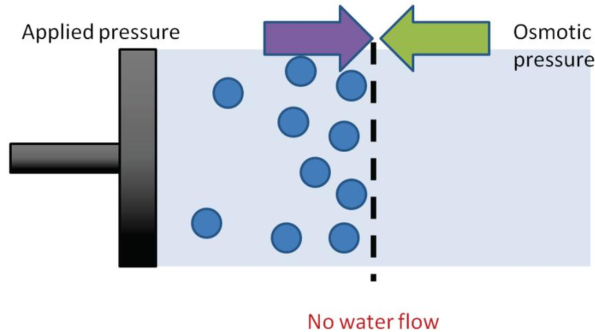
**Figure 11.3:** As the water is forced through, the ions get left behind on the salty side. This means that there will be layer of water with a high concentration of salt next to the membrane. The osmotic pressure depends on concentration, so as the layer gets more and more concentrated, the osmotic pressure builds up and up until eventually the flow of water stops. To get the water flowing again, either the pressure must be increased or the concentration decreased.
