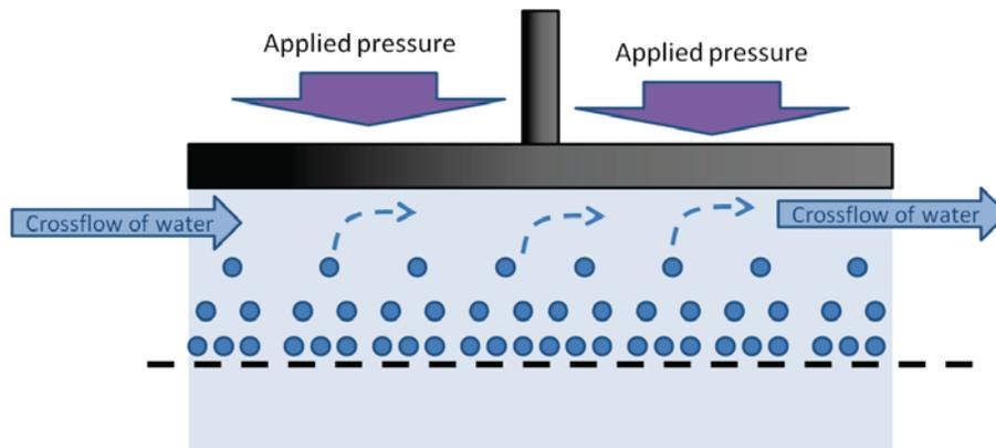
**Figure 11.4:** By introducing water across the membrane, *i.e.* parallel to it, some of the concentration layer can be washed away, thus keeping the osmotic pressure down.
