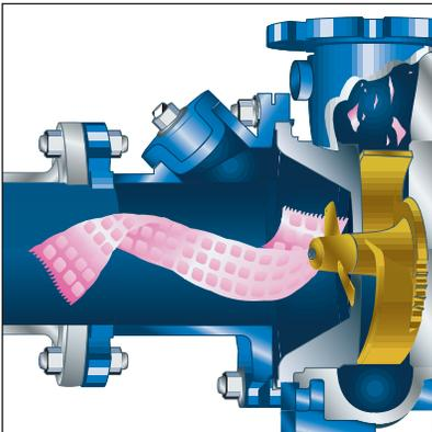
Prior to entering the casing, large solids are chopped and reduced in size to ensure passage through the pump without clogging. An optional disintegrator blade can be added at the inlet to break up large solids and facilitate entry into the suction for further cutting by the impeller.
