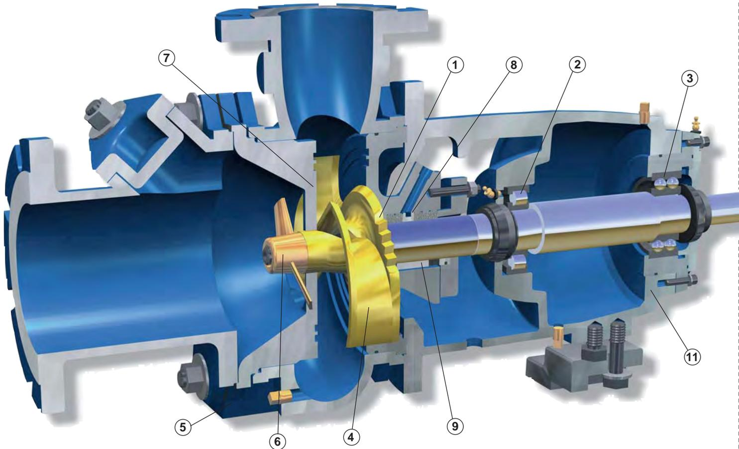
1. Sharpened and serrated patented rear cutter on impeller shroud sweeps over spiral grooves in the casing backplate to cut and then expel stray material from behind the impeller.
