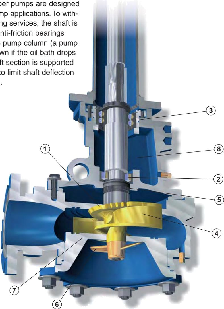
1. Sharpened and serrated patented rear cutter on impeller shroud sweeps over spiral grooves in the casing backplate to cut and then expel stray material from behind the impeller.
